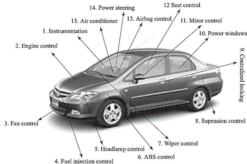
Fig. Embedded system in the automotive domain (Photo courtesy of Honda S16 Car India ( www.hondacarindia.com ))
